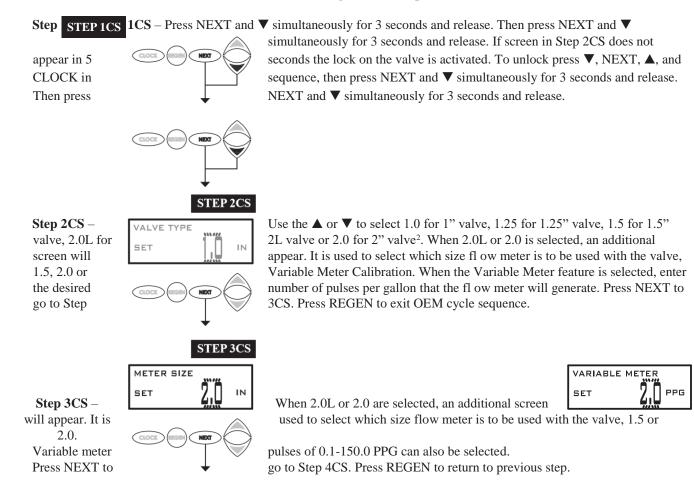
**Note**: When using the WS2 valve, if "2.0L" is set instead of "2.0", when the valve is in regeneration and the piston drives to the "DRAW" cycle the piston will stall and generate a 102 error code. Clear the error code by pressing "NEXT" and "REGEN" buttons simultaneously until the valve resets, then re-program valve to proper valve type setting.
