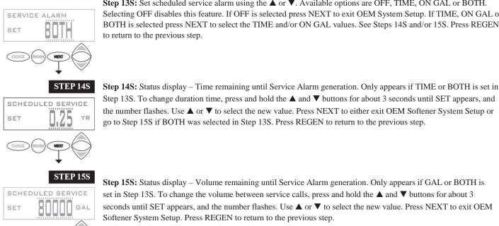
**Step 13S:** Set scheduled service alarm using the  $\blacktriangle$  or  $\blacktriangledown$ . Available options are OFF, TIME, ON GAL or BOTH. Selecting OFF disables this feature. If OFF is selected press NEXT to exit OEM System Setup. If TIME, ON GAL or BOTH is selected press NEXT to select the TIME and/or ON GAL values. See Steps 14S and/or 15S. Press REGEN to return to the previous step.
